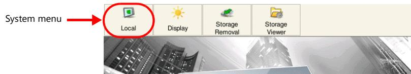
2. Press the [Local] switch on the system menu. The Local mode screen is displayed on the unit.
